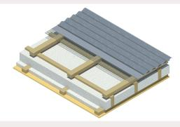
190mm Rafters - Mammoth R3.6 165mm + R1.3 45mm batten insulation or R1.0 35mm batten insulation.
